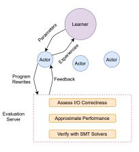
Figure 4: An overview of our actor-learner setup. It features interaction between a centralized learner module, numerous asynchronously-operating actors, as well as a server for evaluating program rewrites.
