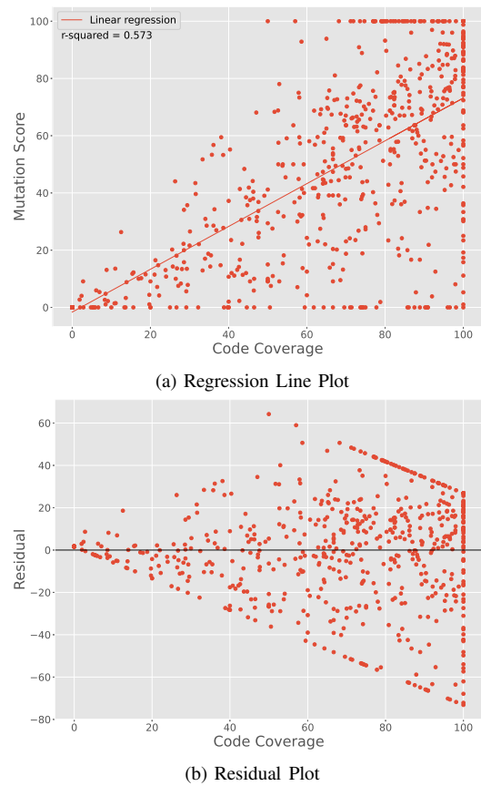
Fig. 1: Regression and residuals of coverage vs mutation score for all lines. Coverage and mutation score are weakly positively correlated.
